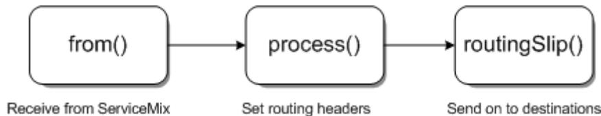
Figure 7. Routing slip implementation in Camel
